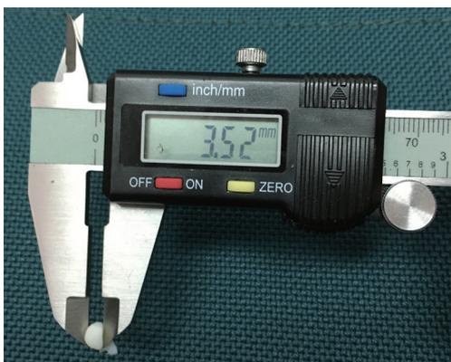
**Figure 5** Use of digital caliper to measure the size of calcification which was inserted into the left main stem of model 1.
