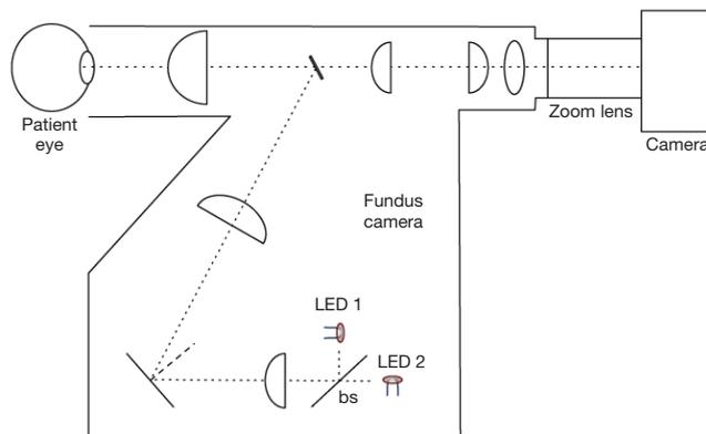
**Figure 1** The layout of the FOS Device. All light sources were replaced with controllable LED systems. The imager consisted of a fundus camera combined with a zoom lens. FOS, Flow Oximetry System; LED, light emitting diode.
