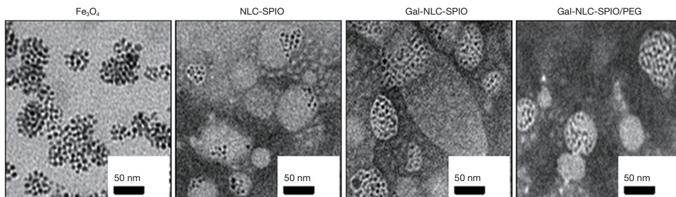
**Figure 2** Preparation and characteristics. TEM images of  $\text{Fe}_3\text{O}_4$ , NLC-SPIO, Gal-NLC-SPIO and Gal-NLC-SPIO/PEG nanoparticles ( $\times 100,000$ , bar = 50 nm). TEM, transmission electron microscopy; Gal-NLC, galactose-conjugated nanostructured lipid carrier; SPIO, superparamagnetic iron oxide.
