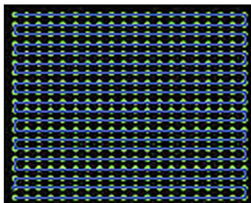
**Figure 4** Pattern of VA imaging scan. The blue line represented the path scanned by the focus of the confocal transducer and the green points the acquisition position. VA, vibro-acoustography.
