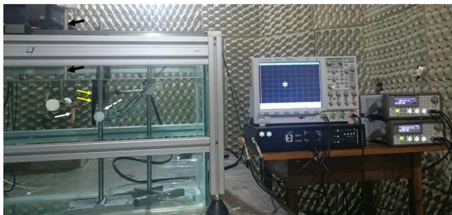
**Figure 1** Acoustic tank where the experiments were made. Black and thick arrows indicate the positioning system. Thin white arrow indicates the femur. White dashed arrow points the confocal transducer. Yellow arrows indicates hydrophone. \*, oscilloscope; \*\*, power amplifier; \*\*\*, function generators.
