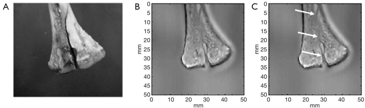
**Figure 5** Bone fracture detection with VA. (A) Photograph of fractured bone. The maximum width of the fracture gap was 2.5 mm; (B) VA-generated image with a 30 kHz beat frequency and a resolution of 0.25 mm; (C) same image of (B) with white arrows indicating the fracture. VA, vibro-acoustography.
