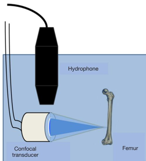
**Figure 2** Experimental setup for VA image generation. The hydrophone was positioned to the side of the confocal transducer and the bone sample was positioned in its focal region. VA, vibro-acoustography.
