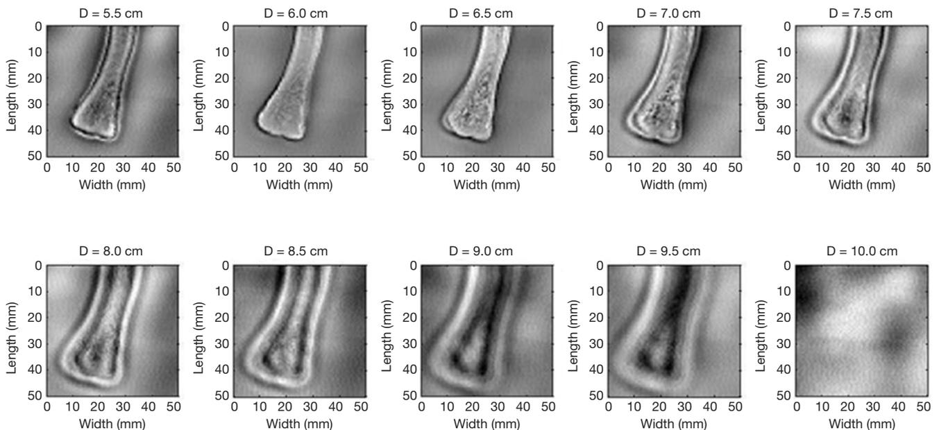
**Figure 6** Series of VA bone images obtained with different distances (D) between the transducer and a bone surface. VA, vibro-acoustography.
