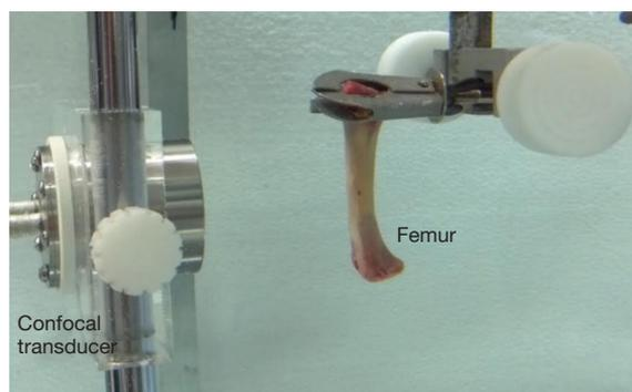
**Figure 3** Placement of the bone sample relative to the confocal transducer.
