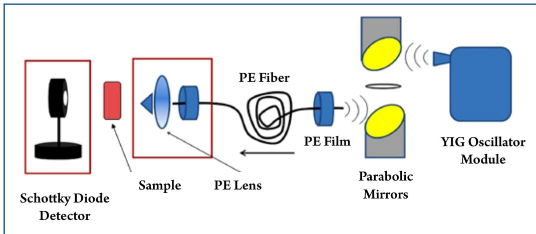
**Figure 3. Schematic illustration of a THz system with transmission geometry using a frequency tuneable oscillator as the THz source and a Schottky diode for detection. PE = polyethylene.**
